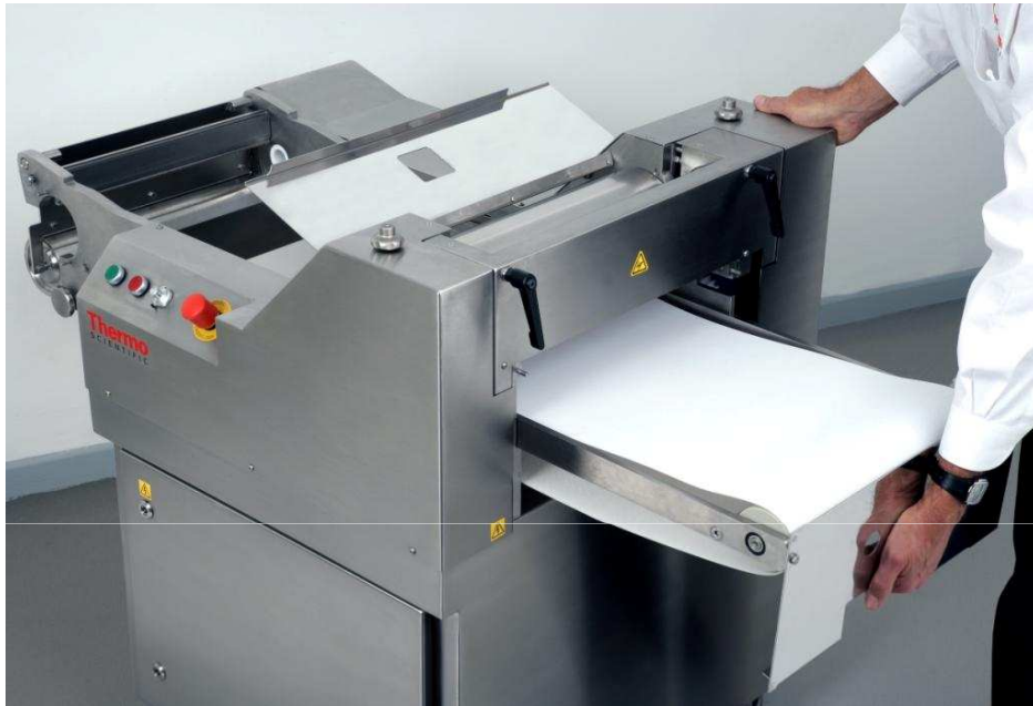
Pharma 24 Chill Roll Removing the Belt Cartridge.
