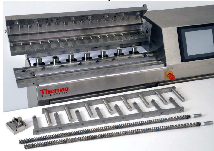
All contact parts removed
