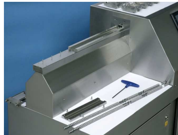
Lower liner and screws removed
