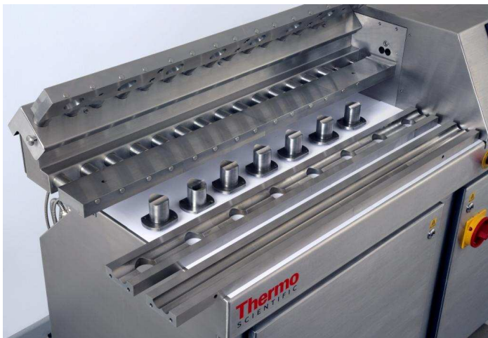
Barrel liners and plugs removed
